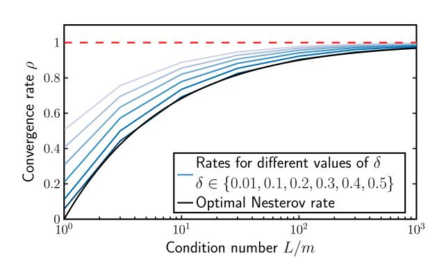
Robustness recovered by designing  $(\alpha, \beta_1, \beta_2)$  in a new algorithm:  $x_{k+1} = x_k - \alpha \nabla f(x_k + \beta_1(x_k - x_{k-1})) + \beta_2(x_k - x_{k-1})$
