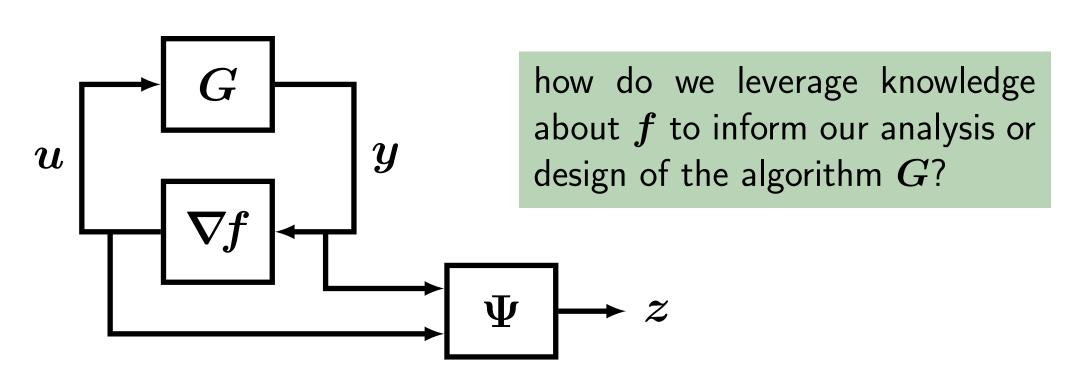
G: discrete-time linear dynamical system (the iterative algorithm)
