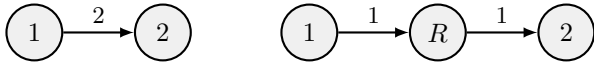
Figure 5: Network graph for a two-timestep delay. The equivalent representation on the right uses a relay node and two one-timestep delays.
