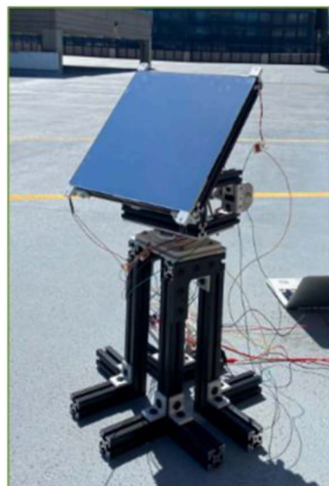
Fig. 11 Closed-loop heliostat system
