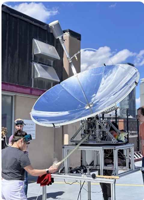
Fig. 13 Solar pyrolyzer dish
