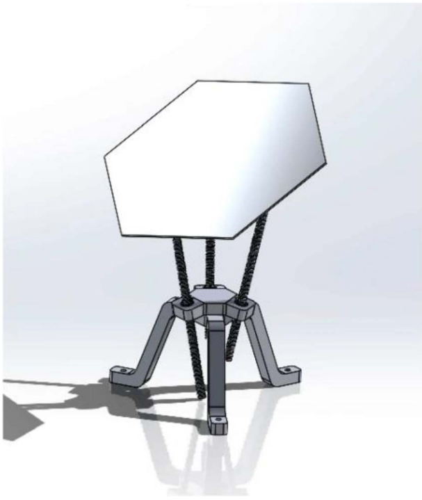
Fig. 7 Second heliostat project assembly
